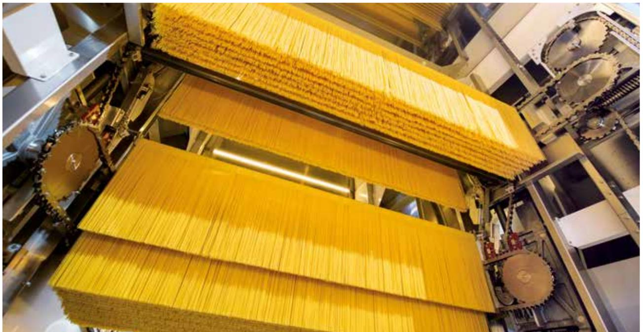
The Bühler Ecothermatik pasta dryer uses 40% less thermal energy.
